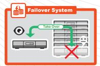
A proportion of FOS NVRs will be assigned as failover servers to the whole surveillance system. Usually 1 FOS NVR shall be worked with 7 NVRs. When any of the NVRs is down, the FOS NVR will soon take over all the works the NVR was doing to keep the whole system working properly. Users could be notified of this take-over event by checking the health check on CMS, and take necessary actions.
