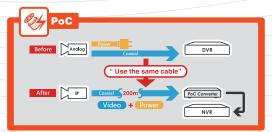
PoC, power-over-coaxial, is a technology to transfer power and video signals via one coaxial cable per camera, eliminating the need to arrange power adapters additionally. For HD IP system upgrade projects, this technology also save the cost to replace existing coaxial cables with network cables. The existing coaxial cables could remain.
