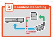
When the NVR and IP cameras are disconnected, the recording task will switch to the cameras, and the recordings are saved to the microSD cards of the cameras. When the NVR and IP cameras are re-connected, the recordings saved in the microSD cards will transfer to the NVR and save in the hard disks without changing the original recordng time. Users could still search the recordings they want by time on the NVR.
