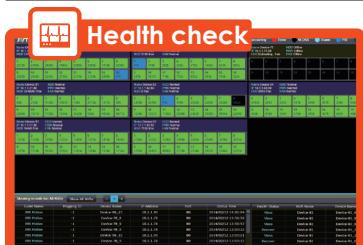
The CMS software shows the status of each connected device in graphic and monitors all the time in case of any abnormal event occurs, maximizing the efficiency of system maintenance.
